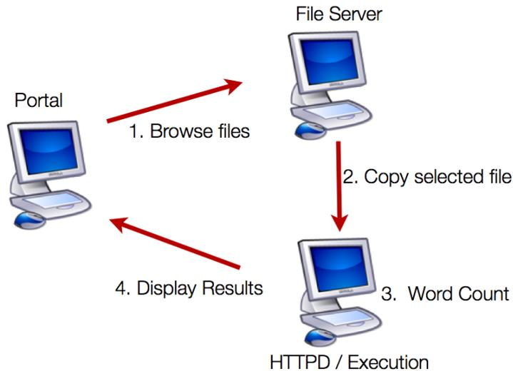
Figure 8: Browsing a remote file system, selecting and copying a file, then executing Unix' word count program and displaying the result directly in the portal
